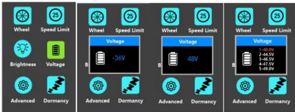
Battery Voltage Settings Interface
